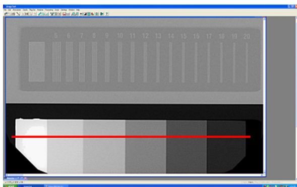
Fig. 8. Computer screen image indicating line profile for dynamic range analysis. Image is available in color at www.ooooe.net .
