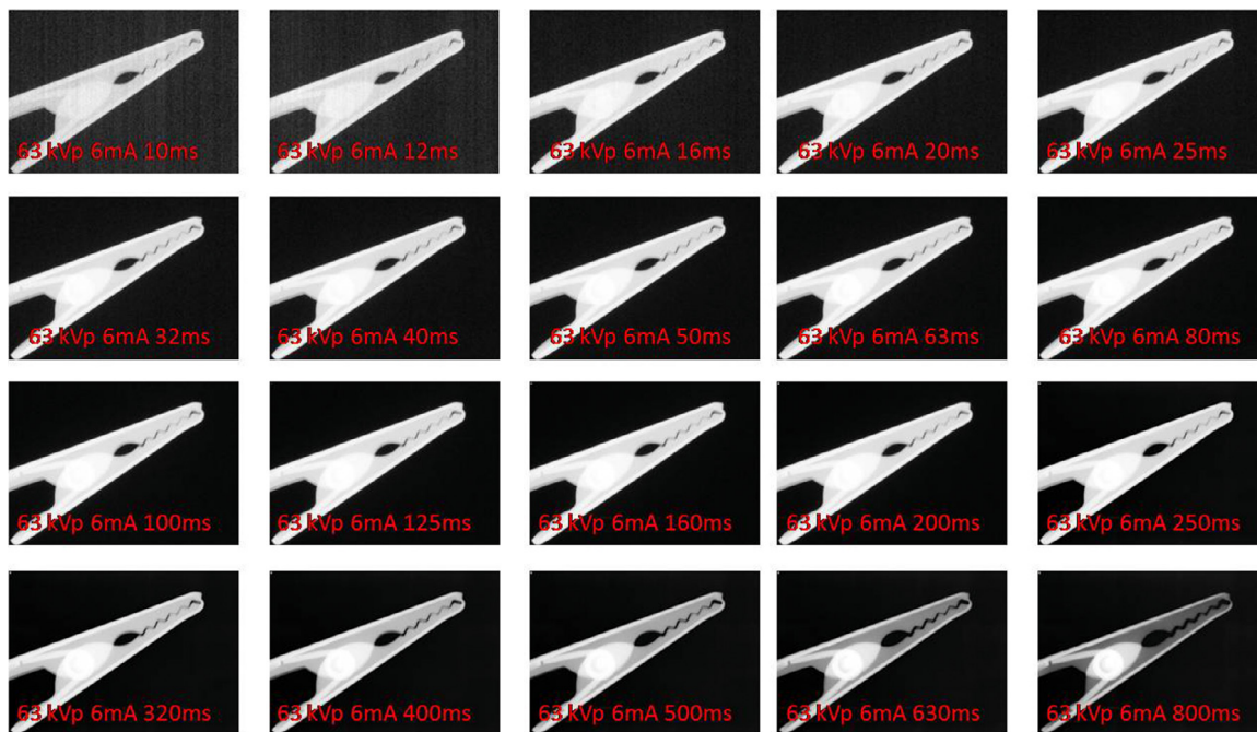
Fig. 4. Radiographs of an alligator clip at incrementally increasing exposures over a range of 20 exposures. kVp , kilovoltage peak; mA , milliamperes; ms , milliseconds.
